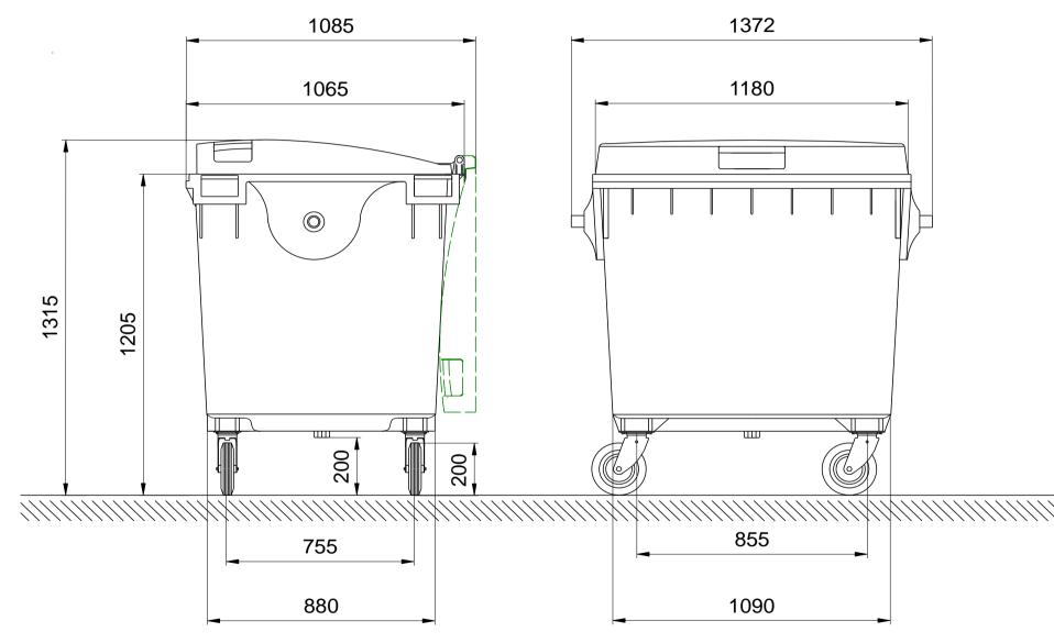
Mobile Waste Containers MGB 1100 Liter Flat Lid Sizes and Measures: Hight 1315 mm<sup>.</sup> Width 1372 mm<sup>.</sup> Depth 1065 mm We reserve the right to make any dimensional and constructional alterations at any time. Dimensions can vary slightly after manufacture.
