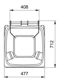
Mobile Garbage Bins MGB 180 Litre Sizes, Measures, Dimensions: Hight 1063 mm; Width 477 mm; Depth 712 mm
