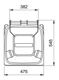
Mobile Garbage Bins MGB 120 Litre Sizes, Measures, Dimensions: Hight 930 mm; Width 475 mm; Depth 545 mm We reserve the right to make any dimensional and constructional alterations at any time. Dimensions can vary slightly after manufacture.
